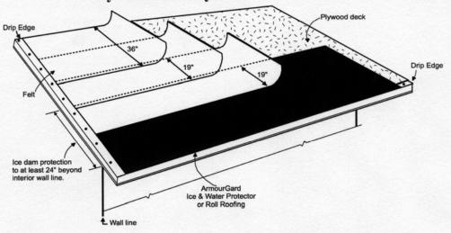
Option C - Cemented Felt Eave Protection and 2-Ply Felt Underlayment
