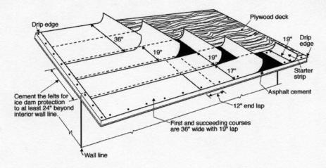
Option D - Applying 3-Tab Shingles for Triple Coverage
