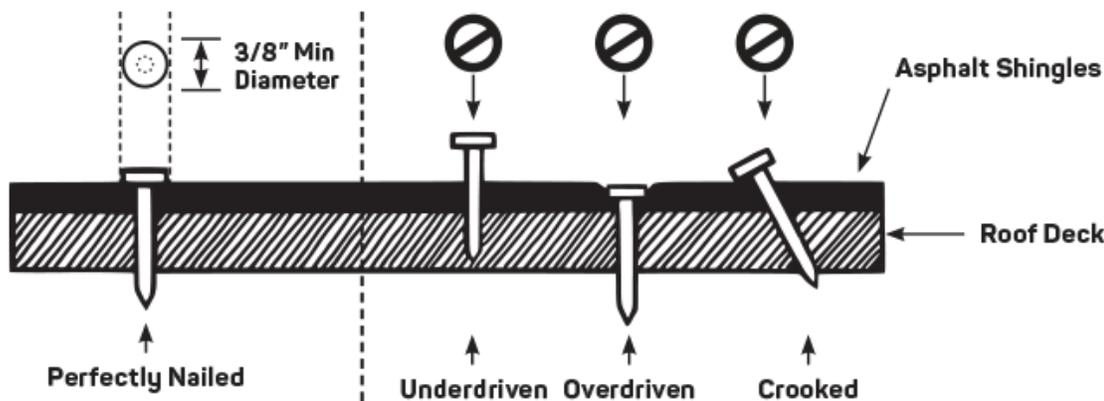
**STEP 9: INSTALL THE FIRST COURSE:** Start with a full length shingle applied flush with starter course at rake and eave. Use four nails per shingle placed as shown below. After the first shingle in the course is installed, continue with full length shingles to complete the first course, trimming the last shingle so that it matches the overhang of the starter course below.
