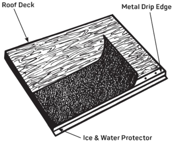
**STEP 4: UNDERLAYMENT:** Apply underlayment, either asphalt saturated felt or synthetic underlayment, such as Stormtite®, in horizontal courses up the roof with 2" side laps and 4" end laps. Trim the sheet to fit the final course at the peak. One layer of asphalt saturated felt (or equivalent) is required over the entire deck to qualify for an ASTM E108 Class A fire rating or which may be required per the local building code.
