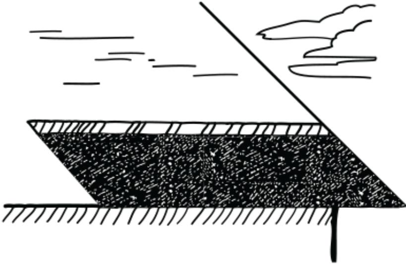
**STEP 10:** End laps must be at least 6" (15 cm) and rolled to ensure adhesion and should be located at least 24" (61 cm) from those in the previous course. If using on a low slope roof (2:12 – 4:12 pitch), cover entire area with CRC's Ice & Water Protector, lapped as outlined above, and then apply shingles matching exposure to the shingles on field of the roof.
