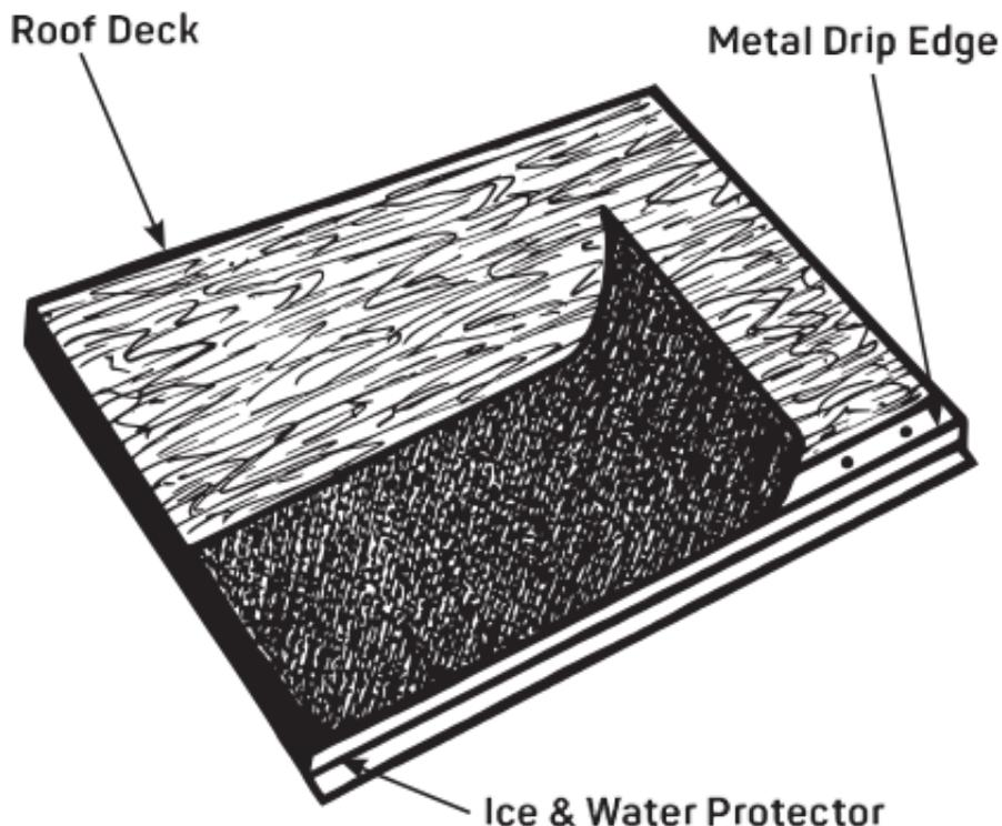
**STEP 4:** Cut the membrane into into 10' (3 m) to 15' (4.5 m) lengths.
