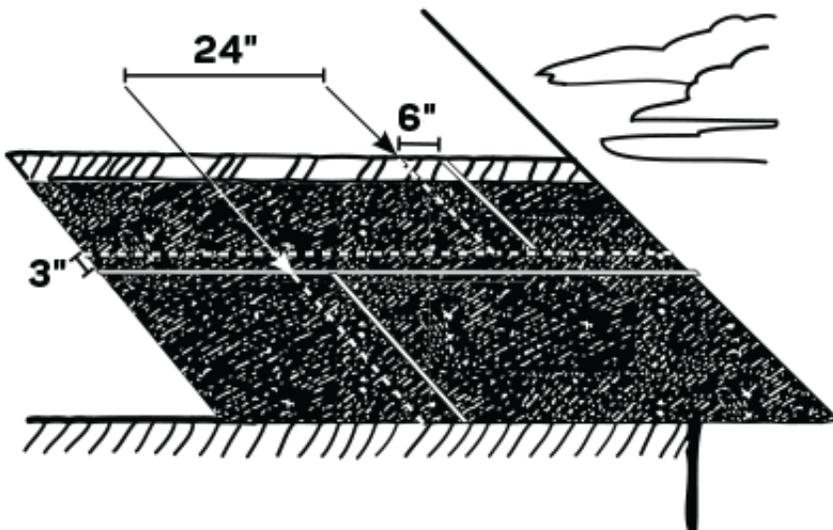
**Valleys and Ridges:** Cut the membrane into 4' (1.2 m) to 6' (1.8 m) lengths. In the valley, start at the low point and work upwards, overlapping each sheet at least 6" (15 cm). Peel off the release film and center the sheet over the valley or ridge. Drape and press in place working from the center outward toward the edges. Membranes must not be left exposed in an open valley.
