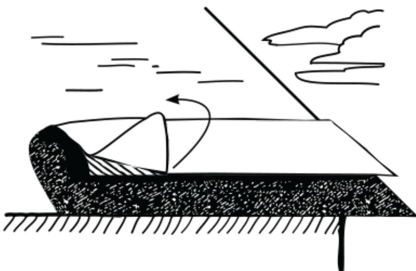
**STEP 9: Carefully reposition the membrane:** up onto the deck and press firmly in place. Avoid wrinkles. If more than one course is to be used, the top course should overlap the seldge tape on the lower course.
