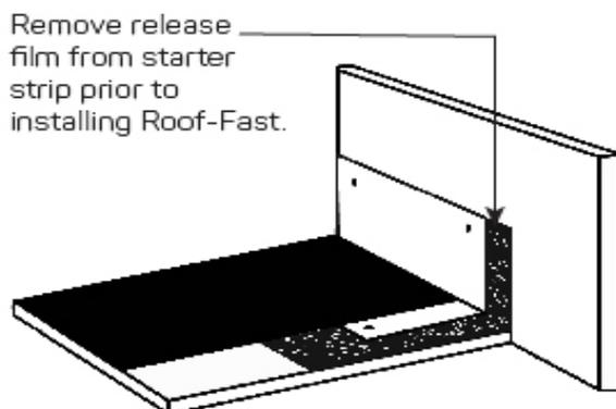
**STEP 18:** After adhering the Roof-Fast 95 Base sheets, it is recommended that uniform pressure be applied to the entire roll area (including overlaps onto metal at roof edges and rakes) by a method suitable to the slope of the roof. A steel or silicone roller would be appropriate at seams and metal overlaps. This is the first layer of the **2-ply** system.
